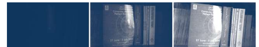
(a) Camera output with ISO 8,000 (b) Camera output with ISO 409,600 (c) Our result from the raw data of (a)
