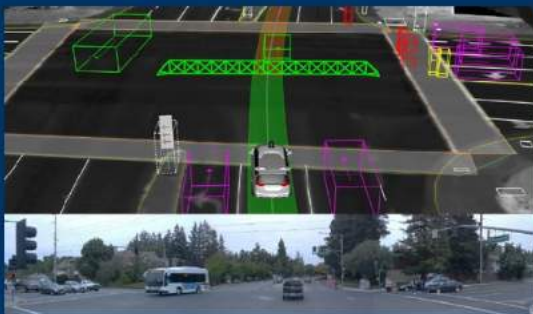
The green path indicates the trajectory through which our vehicle can proceed ahead. The series of green fences indicate that the self-driving vehicle can proceed, and that the vehicle has identified the vehicles ahead and understands it has to maintain certain headway.
