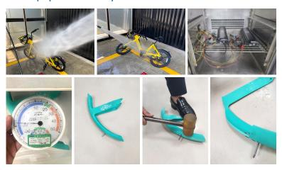
Kakao T Bike applies its own design standards that go beyond Korea Certification standards from the design stage. Frame and parts durability tests are added, and driving ability evaluation goes beyond simple mileage measurement to create and evaluate comprehensive indicators such as ride comfort, fatigue, and durability.
