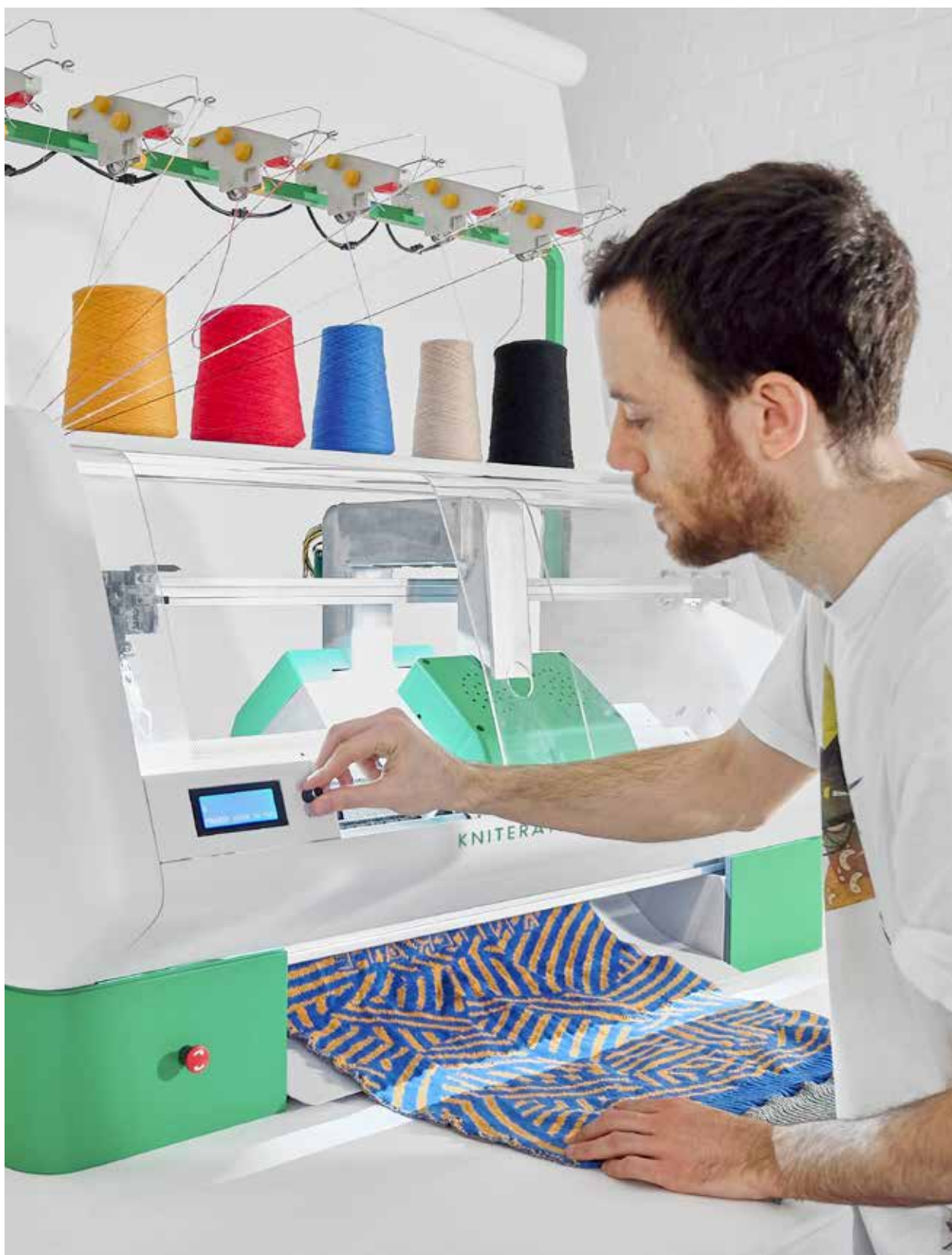
Kniterate is a compact digital knitting machine that brings fashion fabrication into small businesses and design studios, workshops, makerspaces and schools. At the click of a button, it allows users to take a digital design and knit it into a wearable fabric.
