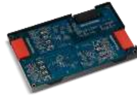
Battery Management System (BMS)
