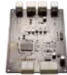
Battery Management System (BMS)
