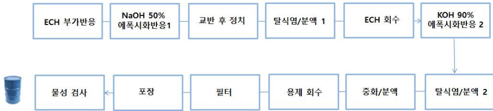
Fig. 6. The expected synthetic process of multi-functional epoxy resin.
