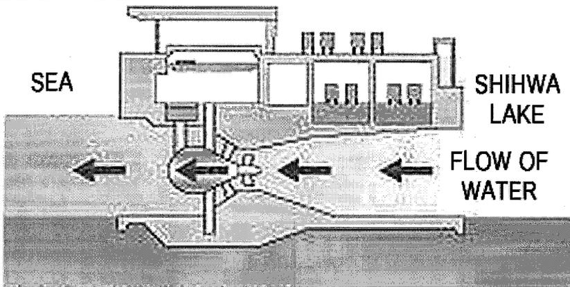
DISCHARGE WATER WITHOUT GENERATING ELECTRIC POWER
