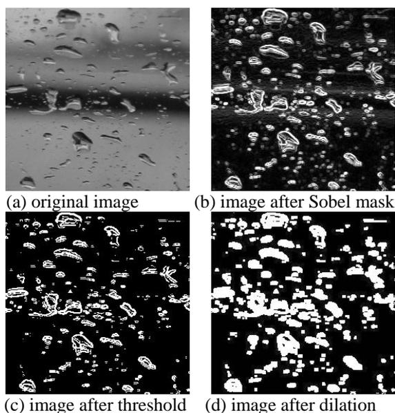
**Fig. 11 Result of image processing for rain in the daytime**
