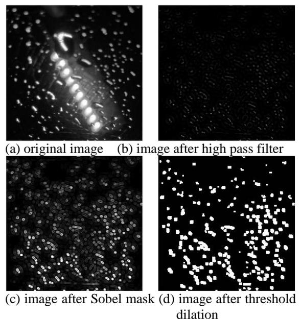
**Fig. 13 Result of image processing for rain in the nighttime**
