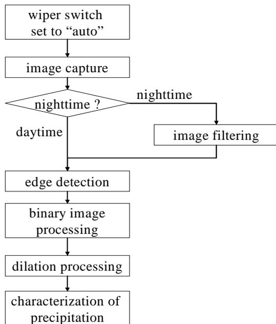
Fig. 3 Flowchart of rain sensing algorithm
