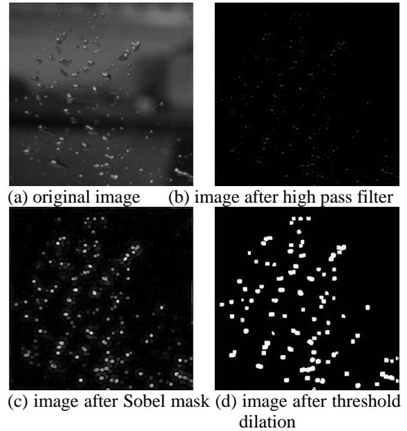
**Fig. 12 Result of image processing for drizzle in the nighttime**
