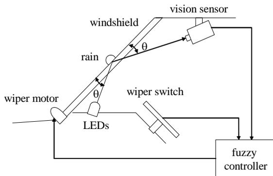
**Fig. 1 Schematic diagram of vision-based smart wiper system**
