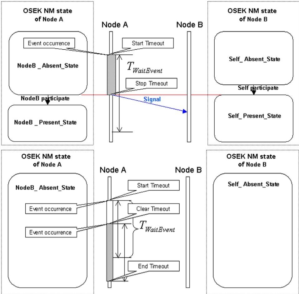
Figure6. Network Fault Countermeasure for Event Signal
