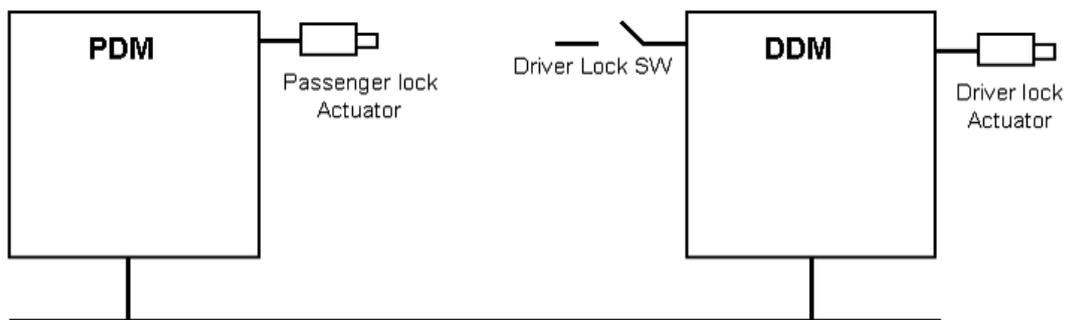
Figure7. Structure of Central Door Lock System
