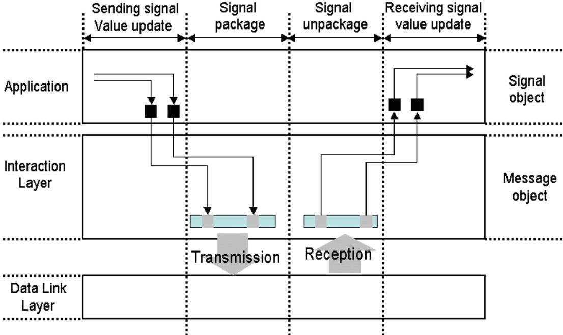
Figure2. Signal-Oriented Interface Using Interaction Layer
