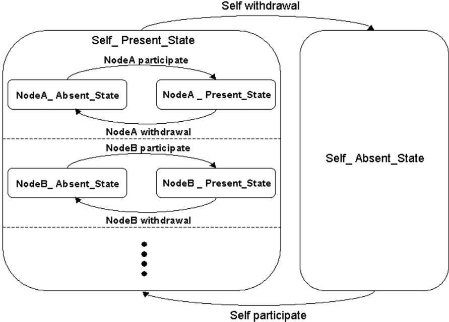
Figure1. The State Diagram of OSEK-NM Design Attributes
