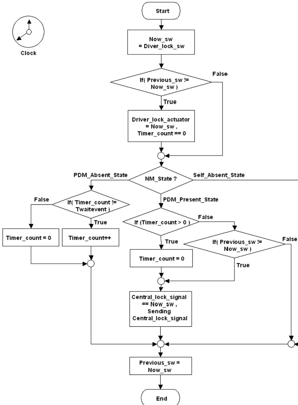
Figure8. Flowchart of Central Door Lock Function in Driver Door Module
