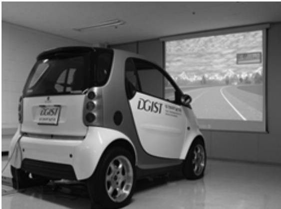
**Figure 1. The DGIST fixed-based driving simulator**
