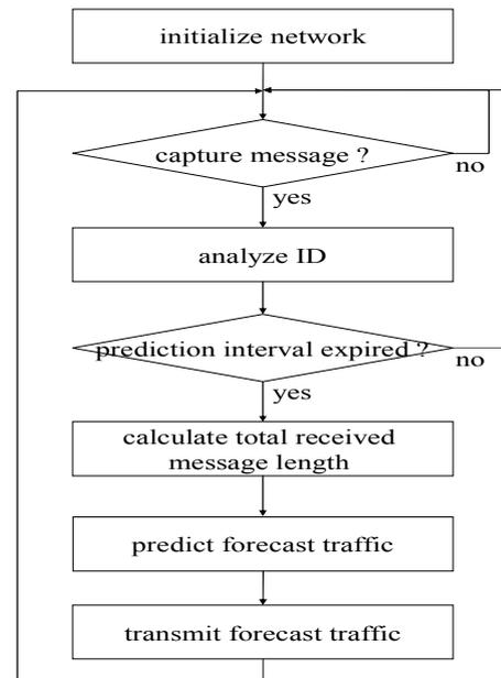
Fig. 2 Flowchart of the traffic prediction method used by the traffic prediction node
