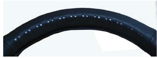
Figure 8. Optical sensors attached on a wheel for ECG signal measurement
