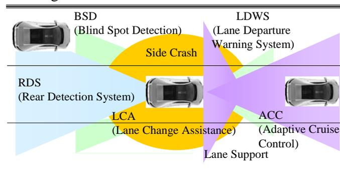
Figure 1: Advanced Driver Assistance System for intelligent vehicles.
