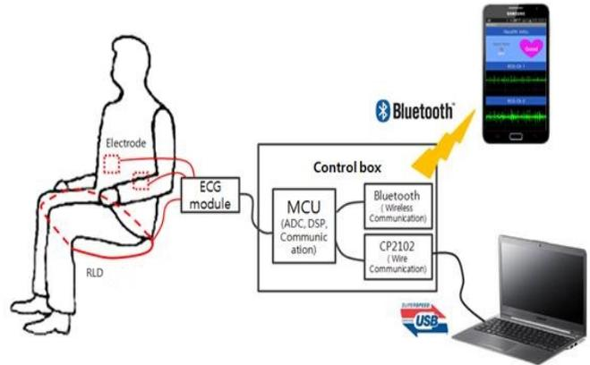
Figure 1. ECG sensing system overview
