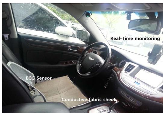
Figure 2. Non-intrusive ECG sensing system
