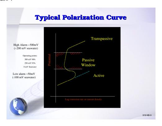
The anodic protection system consists of several reference electrodes, one of which is usually the controlling electrode. The system measures the potential of the wetted surfaces and feeds the information to the controller. The controller regulates the amount of current supplied by the power supply through the cathodes to maintain the system with the passive window.
