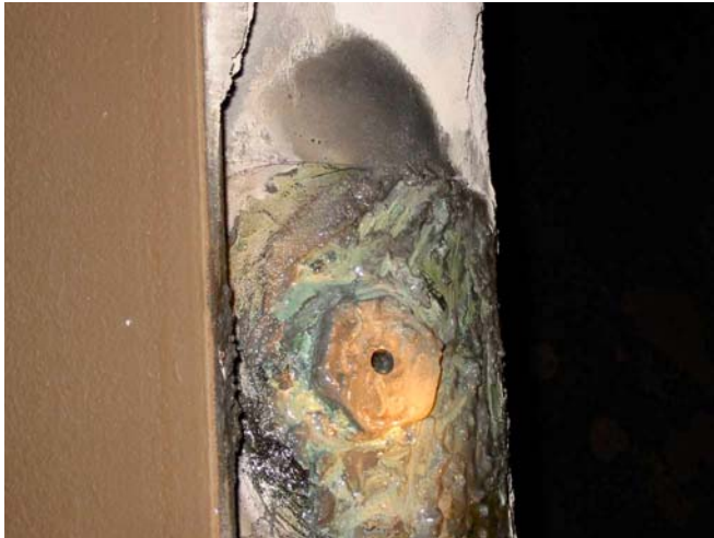
Figure 4: Sulfuric Acid Deposits on Injector nozzle due to cold operation less than 232 °C
