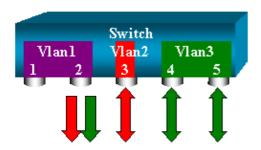
With the above configuration, every single packet entering or leaving VLAN 2 or 3 will be duplicated to port 6/2. Note that the result is exactly the same as if you were implementing SPAN individually on all the ports belonging to the VLANs specified in the command. You can see this by comparing the **Oper Source** and the **Admin Source** fields. The Admin Source basically lists all that you have configured for the SPAN session, whereas the Oper Source field lists what ports are using SPAN.
