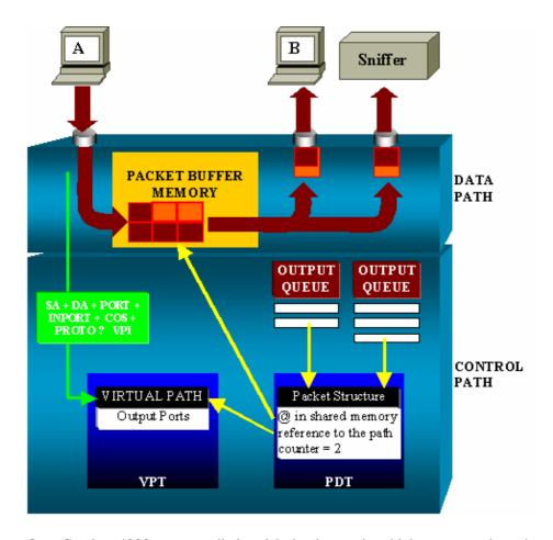
On a Catalyst 4000, you can distinguish the data path, which corresponds to the real transfer of data within the switch, from the control path, where all the decisions are taken.
