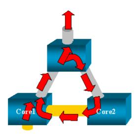
Since the introduction of the inpkts (input packets) option on the CatOS, a SPAN destination port drops by default any incoming packets, thus preventing this failure scenario. But the potential issue is still present on the Catalyst 2900XL/3500XL family. Note also that even with the inpkts option preventing the loop, the above configuration could cause some problem in the network (because of the learning enabled on the destination port at least).
