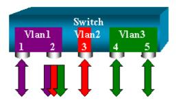
The **set span** *source ports destination port* allows the user to specify more than one source port. Just list all the ports on which you want to implement the SPAN, separated by commas. The command line interpreter also allows you to specify a range of ports by using the hyphen. The following example illustrates this ability: SPAN on port 6/1 and a range of three ports starting from 6/3 is used. There can only be one destination port, and it is always specified after the SPAN source.
