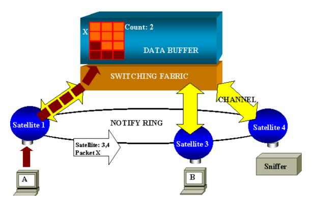
The ports of the switch are attached to satellites that communicate to a switching fabric via radial channels. On the top of that, all the satellites are interconnected via a high–speed notify ring, dedicated to signaling traffic.
