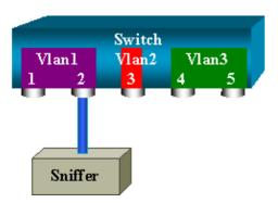
This diagram represents part of a single line card located in slot 6 of a Catalyst 6000 switch. Ports 6/1 and 6/2 belong to VLAN 1, port 6/3 belongs to VLAN 2, and ports 6/4 and 6/5 belong to VLAN 3. Connect a sniffer to port 6/2 and use it as a monitor port in several different cases.
