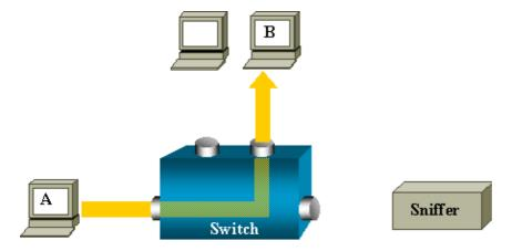
In this configuration, the sniffer would only capture traffic flooded to all ports like broadcast traffic, multicast traffic with CGMP or IGMP snooping disabled and unknown unicast traffic. Unicast flooding happens when the switch does not have the destination MAC in its CAM table. It will not know where to send the traffic and it will flood the packets to all the ports in the destination VLAN.
