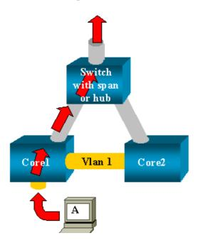
Two core switches, linked by a trunk for instance, each of them having several servers, clients or other bridges connected to them. The administrator wants to monitor VLAN 1 that is appearing on several bridges with SPAN. In order to achieve that, he created a SPAN session monitoring the whole VLAN 1 on each core switch, and, in order to merge these two sessions, the destination port is connected to the same hub (or the same switch, using another SPAN session).
