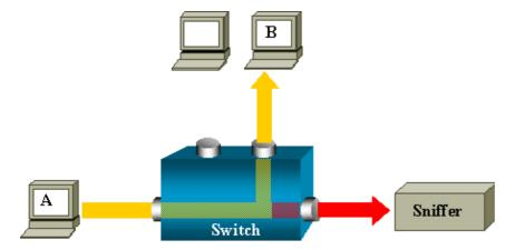
In this above diagram, the sniffer is attached to a port that is configured to receive a copy of every single packet that is sent by host A. This port is called a SPAN port. The sections below describe how this feature can be tuned very precisely to do more than just monitoring a port.
