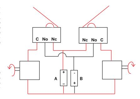
But when the bot hits an obstacle, the switch closes the circuit with the negative-side battery, through the NO terminal. This reverses the motor on that side while the other side continues running forward. The bot turns away from the obstacle.
