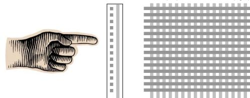
Figure 2. ITO Touch-Screen or PCB Touch-Pad Cross Section (left) and Screen View (right)
