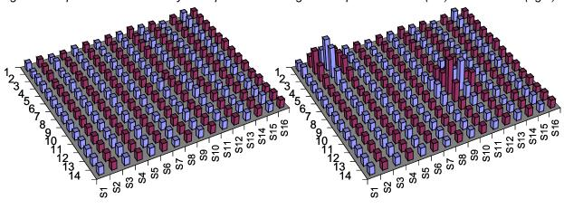
Figure 5. Representative 2D Array of Capacitance-to-Digital Samples: Baseline (left) and Touched (right)
