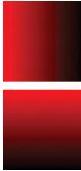
Figure 8-9. A linear gradient before (top) and after (bottom) rotation with the Matrix class
