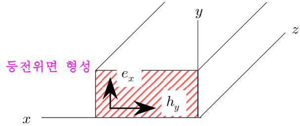
(2) TE 모드(Transverse Electric mode) ; H wave
