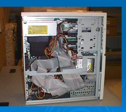
Over a half dozen hard drives!!! Is it a RAID or not? This is important as it can determine *how* to image.
