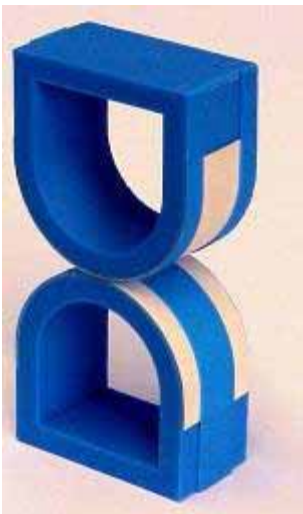
Rolling joint model by Dr. Just Herder of the Delft University of Technology
