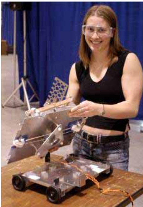
Chandler Hatton used a magnet preloaded kinematic coupling to enable her machine's module to be easily flipped depending which side of the table on which she had to setup
