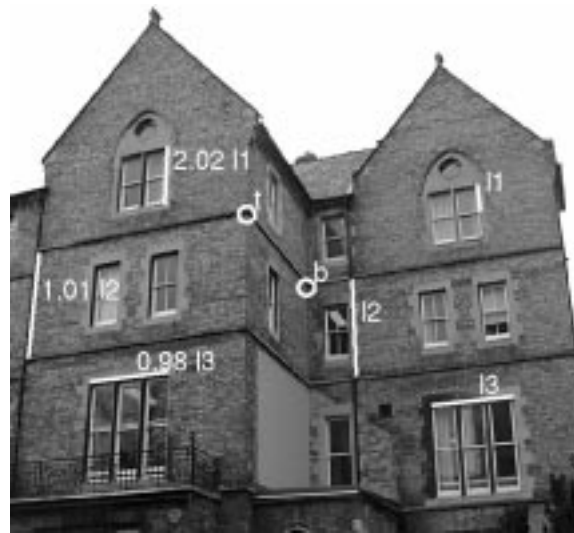
Figure 5: Measuring the ratio of lengths of parallel line segments lying on two parallel scene planes: The points t and b (together with the plane vanishing line and the vanishing point) define the homology between the two planes on the facade of the building.
