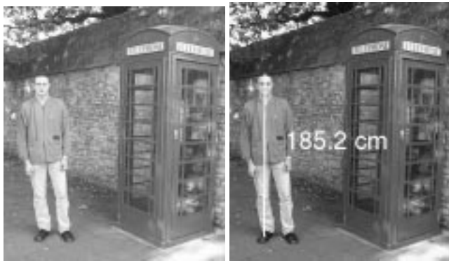
Figure 10: Measuring the height of a person in an outdoor scene: The ground plane is the reference plane, and its vanishing line is computed from the slabs on the floor. The vertical vanishing point is computed from the edges of the phone box, whose height is known and used as reference. The veridical height is 187cm, but note that the person is leaning slightly on his right foot.
