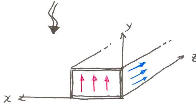
$$(b-28) \quad Z_{TE} = \frac{j\omega\mu}{\beta} = \frac{\omega\mu}{\beta_{10}}$$
