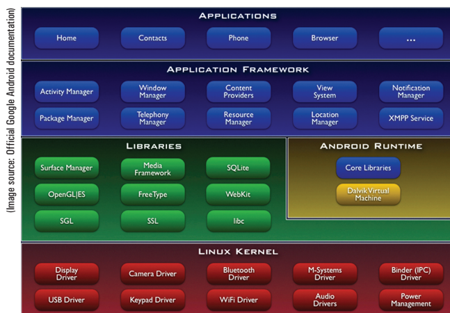
Figure 1: The Android component stack
