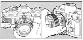
To mount the lens, first align the red positioning point on the lens with the red dot above the camera mount as illus-
