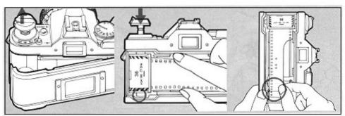
Pull up the rewind knob until the back cover pops open. The AE-1 PROGRAM uses color (negative or slide) or black-and-white film in standard 35mm cartridges. Place the cartridge in the film chamber as shown. Then push the rewind knob down, turning it until it drops into its normal position.
