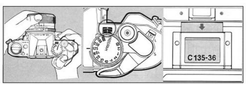
Take several blank shots, releasing the shutter and advancing the film, until the frame counter reads "1." While doing this, keep an eye on the rewind knob. If it rotates in the direction of the arrow, the film is loaded correctly.
