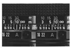
When you load the AE-1 PROGRAM with blackand-white infrared film, it is necessary to make a slight adjustment in focus. A red infrared index is engraved on most Canon lenses for this purpose. First focus as usual through the viewfinder. Then read the distance opposite the distance index on the lens and turn the focusing ring to align that distance with the infrared index. It will also be necessary to use a deep red filter, as specified by the film manufacturer, over the lens.
