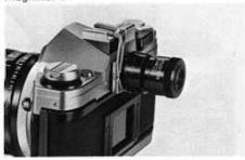
The Magnifier S gives a 2.5X magnification of the center of the viewing area for precision focusing in close-up work and wide-angle photography. Its power is adjustable to your eyesight within a range of +4 to -4 diopters. Its adapter is hinged so that the magnifier can be swung upward from the eyepiece, leaving the entire screen image visible.
