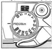
Turn the shutter speed selector dial until "PROGRAM" is aligned with the index.
