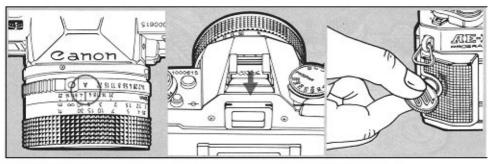
Remove the viewfinder cover from the accessory shoe. Remove the action grip by means of a coin or similar object
