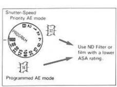
Shutter-speed priority AE mode: When "32" blinks and the shutter speed selector dial is set to 1000; or Programmed AF mode: When "16" blinks
