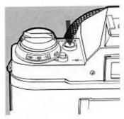
If you have started the selftimer and wish to cancel it before shutter release, press the battery check button or push the main switch back to
