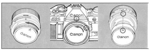
Turn the rear lens cap in the direction of the arrow until it stops and pull it off the lens.
