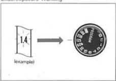
Shutter-speed priority AE mode: A number equal to or smaller than the lens' maximum aperture blinks. Choose a slower shutter speed so that the aperture stops blinking.
