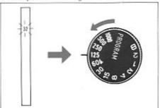
Shutter-speed priority AE mode: "32" blinks regardless of the minimum aperture of the lens in use. Choose a faster shutter speed until the display stops blinking. When using a lens whose minimum aperture is f/22 or f/16, even when "32" does not blink, turn the shutter speed selector dial until a number equal to or smaller than the lens' minimum aperture is displayed.
