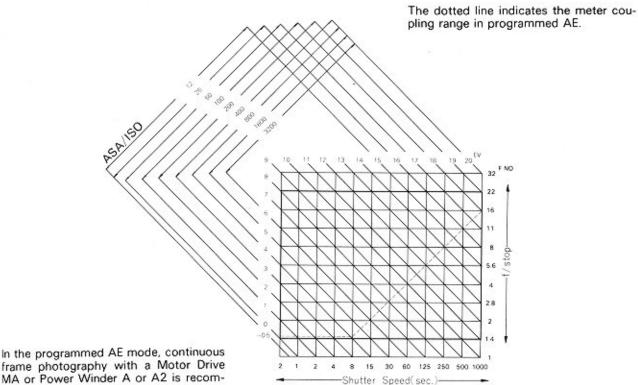
frame photography with a Motor Drive MA or Power Winder A or A2 is recommended only if the light is bright enough to give an aperture display of f/4 or larger. In this case, the shutter speed will be at least 1/60 sec.
