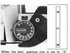
and the shutter speed selector dial to "PROGRAM," a green "P" LED 5 is displayed, indicating programmed AE photography. If the shutter speed selected automatically by the camera is 1/30 sec. or slower, the "P" will blink. This is to warn you that your picture may be blurred due to camera movement if you are
