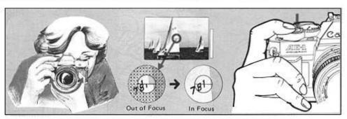
Turn the focusing ring until the main subject is sharp and compose the picture. Gently press the shutter button all the way down to take the picture.
