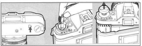
You can tell you have reached the end of the film by the frame counter and the film advance lever. Either the film advance lever will not turn at all or it will not turn all the way. First press in the rewind button.
