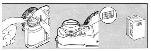
While pressing the lock release button, slide the ASA setting lever until the ASA speed of your film is aligned with the green index. This is necessary for getting correct exposure.
