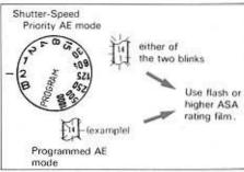
Shutter-speed priority AE mode: When 2 sec. is set on the shutter speed selector dial and a number equal to or smaller than the lens' maximum aperture blinks; or
