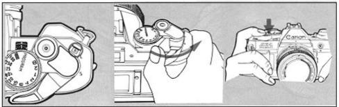
Make sure the main switch is on "A." Turn the film advance lever in the direction of the arrow until it stops. You may turn it in one continuous stroke or in several short strokes. When film is loaded, this will advance it to the next frame. The AE-1 PROGRAM has a two-step shutter button. Press it halfway to turn the meter on and to get a display in the viewfinder. Gently squeeze it all the way down to release the shutter. You cannot release the shutter again until the film is advanced.
