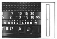
There are two ways to check the depth of field. The usual one is by using the depth-of-field scale on the lens. This is a scale of f/stops repeated on each side of the distance index.
