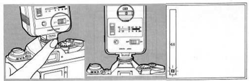
Make sure the main switch on the flash is OFF. Then slide the flash into the AE-1 PRO-GRAM's accessory shoe. Tighten the lock nut. Slide the Speedlite's ASA film speed switch to the ASA speed of your film. Then push the Aperture/MANU selection switch to select an aperture. The green and red positions each indicate the distance range which corresponds to the aperture you have set on the flash.
