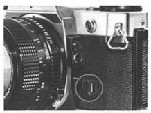
After checking the depth of field, unlock the stop-down lever. Now turn the aperture ring to the smallest number. Then turn it to the largest number, press the AE lock pin and return the aperture ring to "A."
