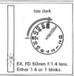
Turn the shutter speed selector dial from "PROGRAM" and set a shutter speed. Refer to the illustrations above when choosing a shutter speed. While looking in the view-finder, press the shutter release button halfway. Exposure will be correct as long as the apperture display does not blink.
