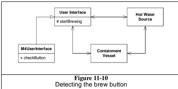
We've derived `M4UserInterface` from `UserInterface`, and we've put a `checkButton()` method in `M4UserInterface`. When this function is called, it will call the `CoffeeMakerAPI.getBrewButtonStatus()` function. If the button has been pressed, it will invoke the protected `startBrewing()` method of `UserInterface`. Listing 11-5 and Listing 11-6 show how this would be coded.
