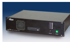
New IPAS10 DGPS/IMU unit developed in-house
