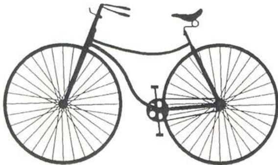
Finally, the pedals were connected to the rear wheel with a chain, the front wheel was returned to a practical size, and a brake was added. This is basically the way a one-speed bicycle remains today. By contrast, early bicycles seem crude and almost useless.
