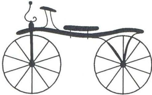
The bicycle is began as a seat on two wheels. The rider's feet pushed to make it go and dragged to make it stop.
