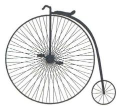
Later, pedals were added to the front wheel was enlarged so that a comfortable rate of pedaling caused the bicycle to go at a reasonable speed.
