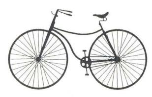
Finally, the pedals were connected to the rear wheel with a chain, the front wheel was returned to a practical size, and a brake was added. This is basically the way a one-speed bicycle remains today. By contrast, early bicycles seem crude and almost useless.
