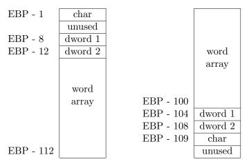
Figure 5.2: Arrangements of the stack
