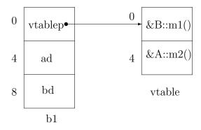
Figure 7.24: Internal representation of b1
