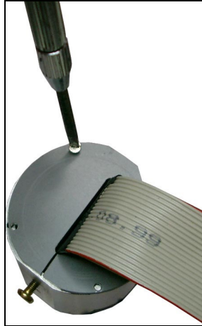
Figure 8 - Securing the housing seal
