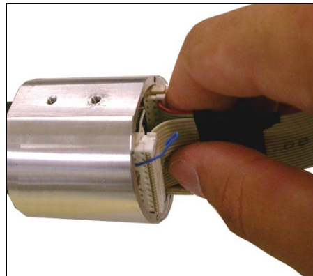
Figure 6 - Inserting the camera board into the housing
