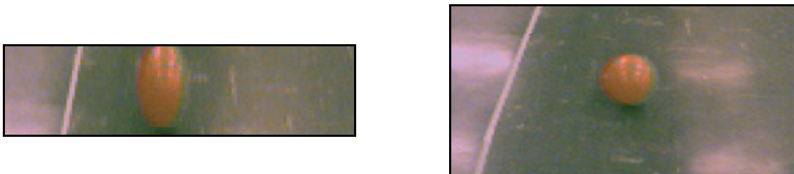
Figure 11 - Initial Resolution (256 x 64) vs Improved Resolution (128 x 128)
