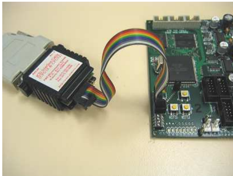
Figure 2.18: ICD Programmer - In System Programming.
