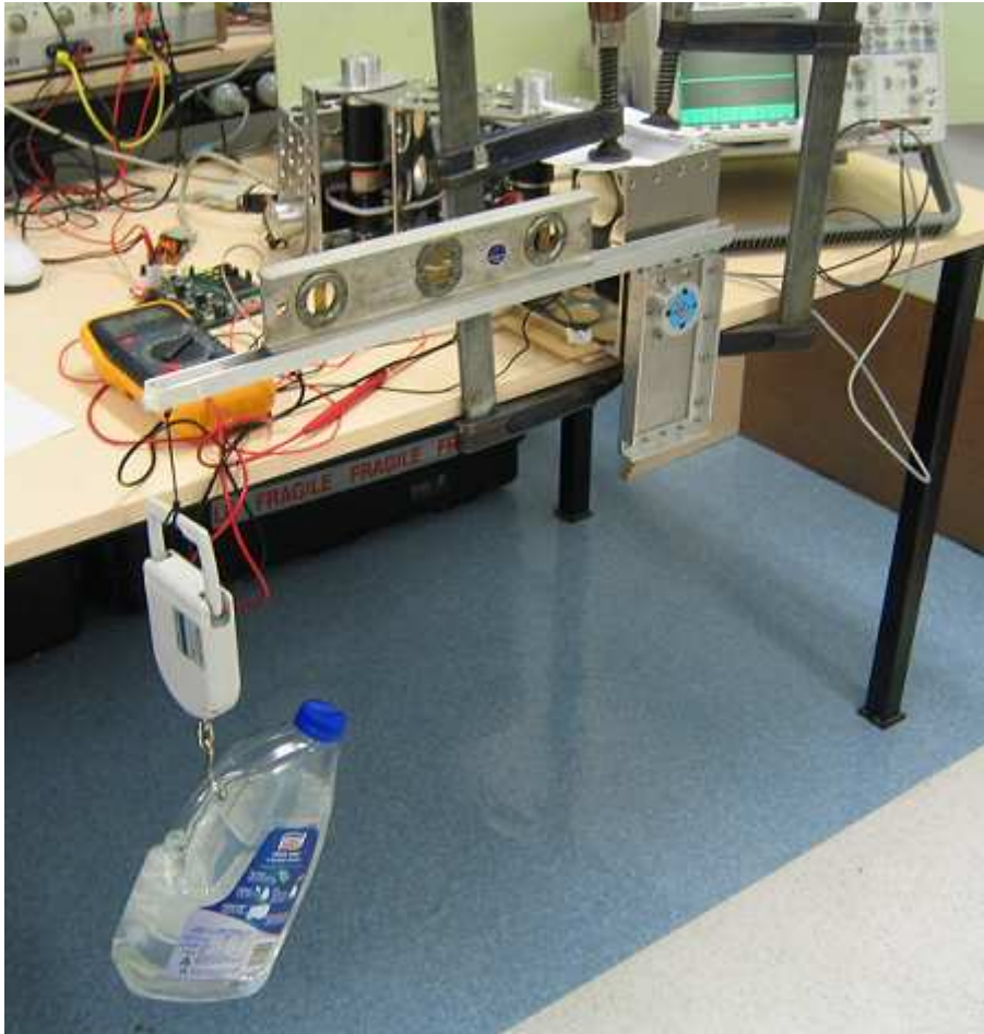
Figure 3.12: Attempted Current Sensing and Torque Correlation Test Apparatus.
