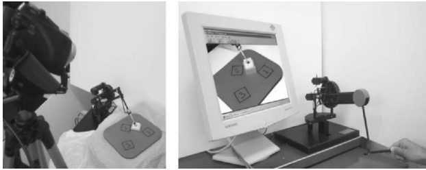
Figure 1. Experimental setup for teleoperation tasks using two PHANTOM haptic interfaces.
