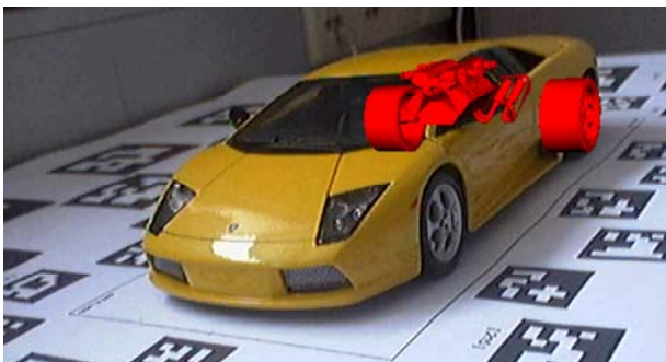
Figure 9 A naïve overlay of hidden information. The engine and the wheels of the car do not provide sufficient depth cues. Ocluded objects seem to be in front of the car rather than inside
