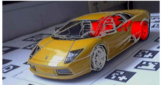
Figure 11 An example of the removal of fragments during Buffer Rendering. This is supported by grouping objects and using OpenGL fragment testing. In the image we combine all the car's faces and the seats. Extracted key features are no longer distracting. This is achieved by displaying only those key features which are visible in the real world's imagery. This yields to a more pleasant and better informative augmentation
