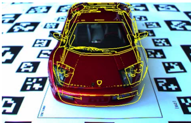
Figure 17 An image showing an augmentation of edges extracted from a 3D model. The edges are thin and clear, however, they suffer from poor registration
