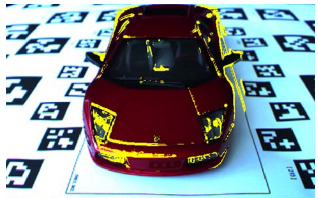
Figure 19 Using the footprint of the model as a mask leads to a less cluttered augmentation of edges from the video stream
