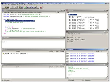
**NOTE** Source and Assembly panes display the main.c program and code.
