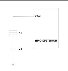
FIGURE 9-2: ASK CRYSTAL CIRCUIT
