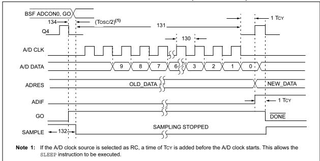
FIGURE 13-10: rfPIC12F675 A/D CONVERSION TIMING (NORMAL MODE)
