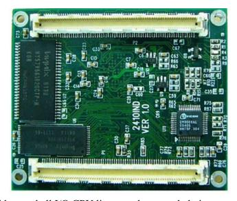
(DM9000AE), IIS, I2C, RTC, PWM, GPIO, Local bus and all I/O CPU lines can be extended via two 4mm height 0.6mm space 140-pin board-to-board connectors. The fully expansion can be used adapted to customer requirements.
