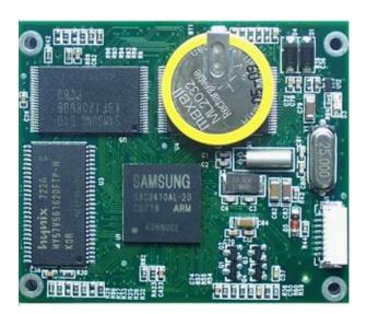
Ethernet (DM9000AE),IIS,I2C,RTC,PWM,GPIO,Local bus and all I/O CPU lines can be extended via two 4mm height 0.6mm space 140-pin board-to-board connectors.
