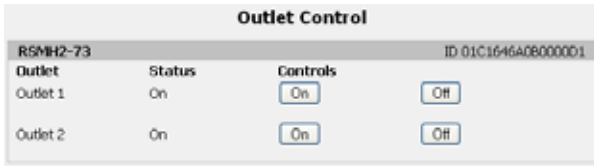
A simple interface to turn on/off a power receptacle.
