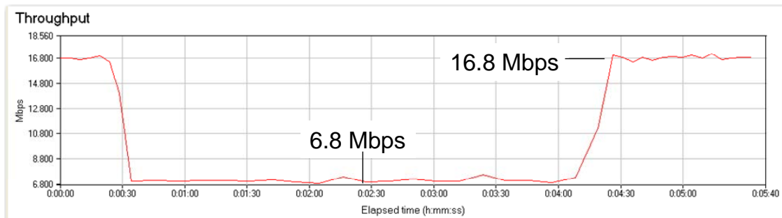
Figure 9: Toshiba throughput over the WiMedia link between the port replicator and the laptop. This test started with the IxChariot TCP/IP throughput via the Gigabit Ethernet port and then a USB file transfer was initiated over the USB port. The IxChariot plot shows the throughput on the Gigabit Ethernet port dropping from 16.8 Mbps when operating alone to 6.8 Mbps when operating in conjunction with the USB port transferring a file.
