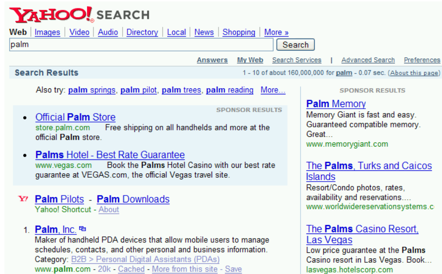
► Figure 9.6 An example of query expansion in the interface of the Yahoo! web search engine in 2006. The expanded query suggestions appear just below the “Search Results” bar.
