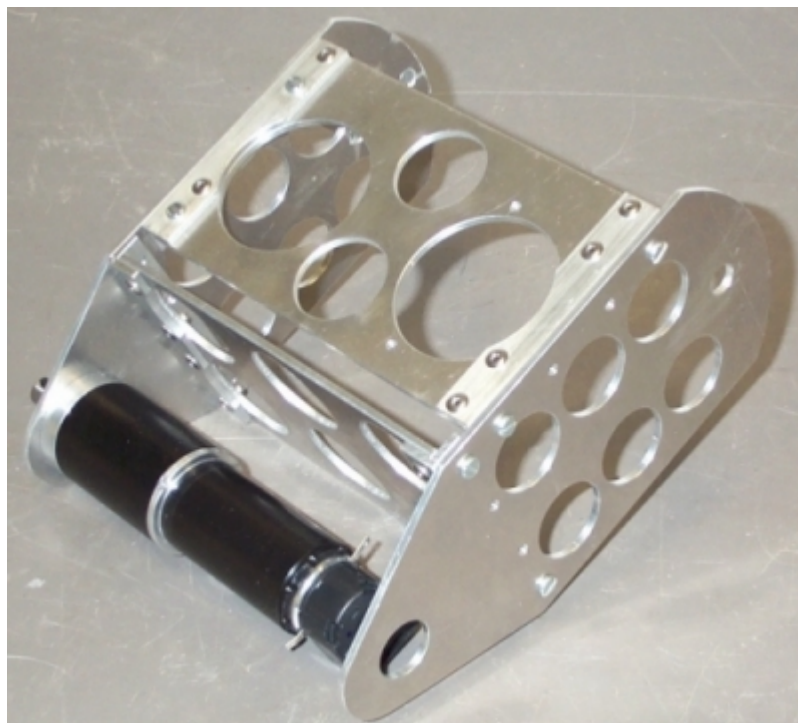
Figure 7.1: Motor within Lower Leg Section
