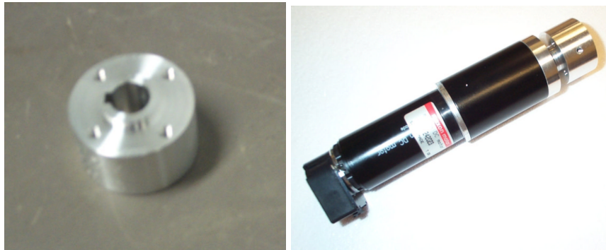
Figure 4.11: Boss and End Cap Assembly with Maxon Motor
