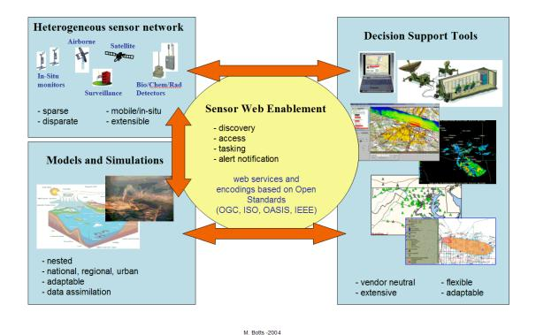
Figure 2: The role of the Sensor Web Enablement framework
