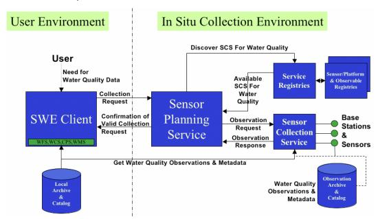
Figure 5: Typical in situ Sensor Planning Service
