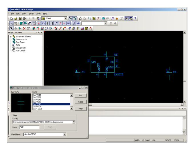
Now select CAP1206 from the Add Part window, press Add and close the window. Before adding the capacitor to your design, press **Ctrl + R** to rotate it 90 degrees. Place the capacitor to the right of the LM2675 as shown below.
