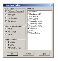
Check the Value checkbox on the right side to enable display of the capacitor's value. Press OK to close the Part Text Visibility window and then press Close to close the Part Properties window. Your schematic should now look like the one below.
