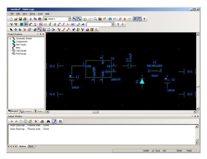
Continue adding connections until your schematic is fully connected as shown below.
