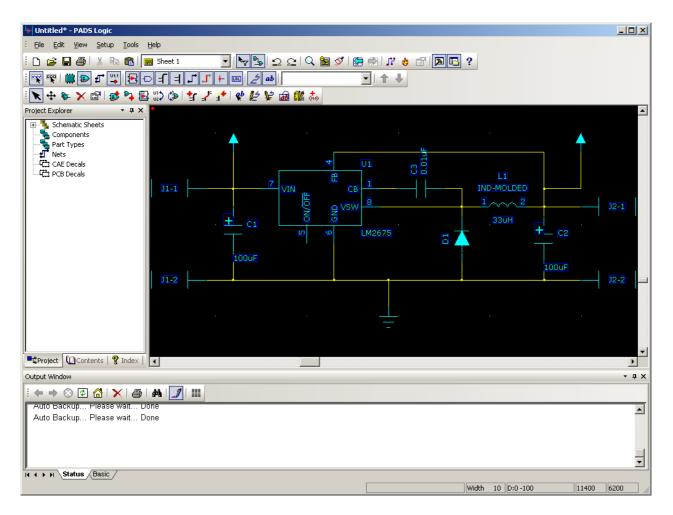
By default, all power connections are automatically connected to a net named +5V. We will need to change this for our design.
