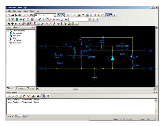
Adding a power connection is done in a similar manner. Begin by starting a new connection from the net connected to pin 7 of the LM2675 and moving up. Right click and select Power from the context menu. Position the power symbol and click once to place it. Repeat this process for the net connected to the top right header pin. Your schematic should look like the one below.
