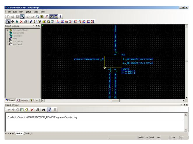
Note: You may wish to zoom in on the decal while making changes to the pins. To enter zoom mode, press **Ctrl + w**. Use the left mouse button to zoom in and the right mouse button to zoom out. Press Esc to exit zoom mode.
