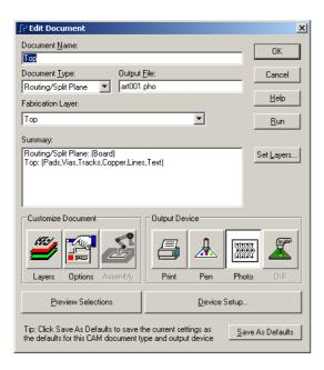
Press the **Device Setup** button to display the Photo Plotter Setup window.
