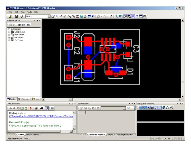
3.5 Save your design. Select **File > Save** and then close PADS Router, returning to PADS Logic. Close the PADS Router Link dialog if it is still open.
