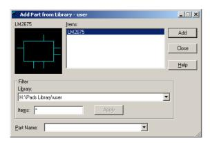
Press the Add button. An outline of the LM2675 part will appear below the mouse pointer while it is within the design window. Close the Add Part window and click somewhere near the center of the sheet to add an instance of the LM2675 part. Press escape to exit add part mode. You schematic window should look similar to the one below.
