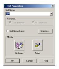
Change the Net Name field to +12V and select the Net Name Label check box. Press OK. Repeat this process for the right power symbol, setting the Net Name to +3.3V. The completed schematic should look similar to the image shown below.
