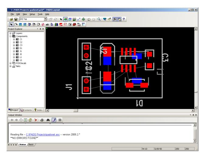
Note: You may need to resize the placement grid to fit all of the parts on the board. Use the modeless grid command, G, to resize the grid. Ex: type **g** 50 to set the grid interval to 50 mils.
