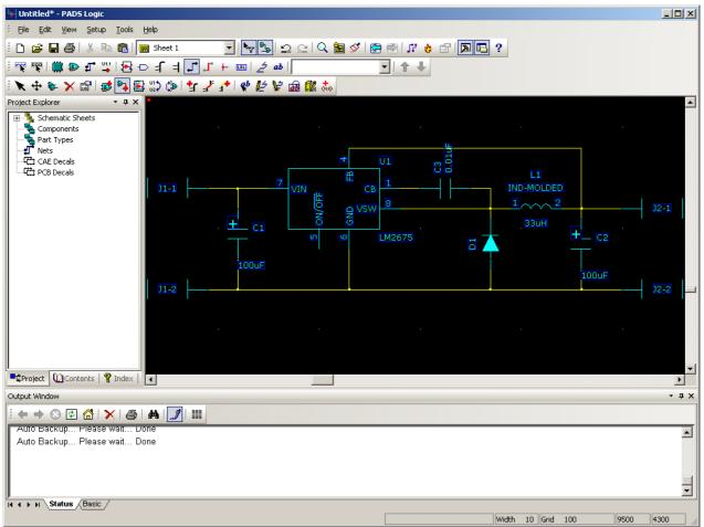
Note: To remove a misplaced connection, ensure that the selection filter allows selecting connections. Then click on the connection you wish to remove and press delete. You can also activate Delete Mode by pressing the 🗙 button on the design toolbar. This will allow you to remove objects with a single click.
