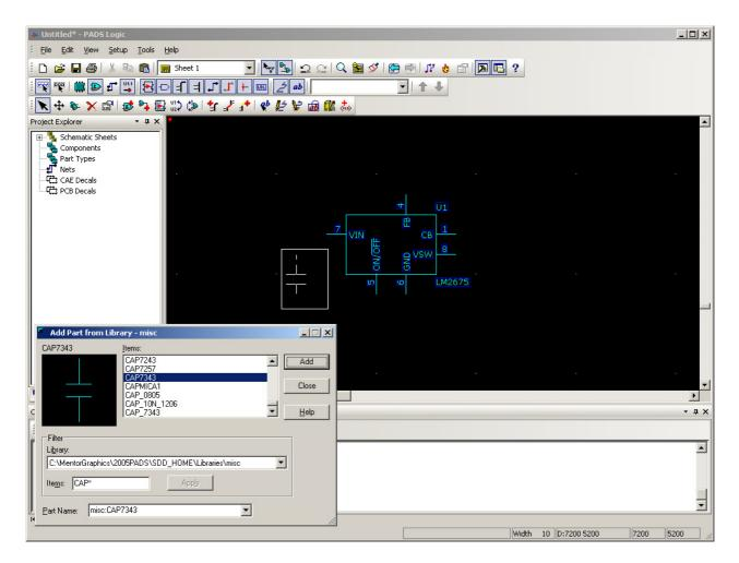
Place the CAP7343 capacitor to the left of the LM2675 as shown above. Place a second CAP7343 to the far right as shown in the schematic below.
