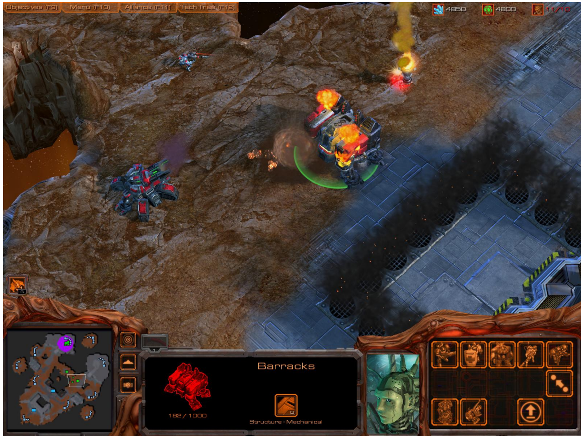
Figure 16. Translucent shadows allow objects such as smoke and explosion to cast shadows.
