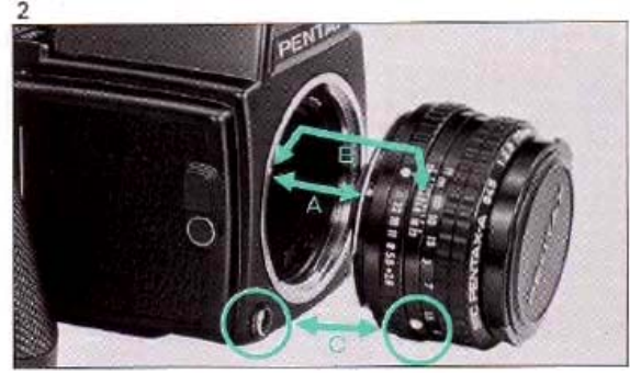
2. To mount the lens, align red dot (A) found on the camera body with red dot (B) on the lens unit, then seat the lens mount into the camera mounting. Turn clockwise until the lens locks with a click.
