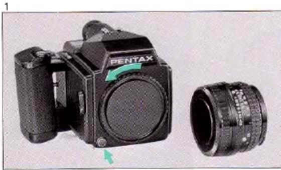
1. Depress the lens release button and turn the body mount cap to remove it.
