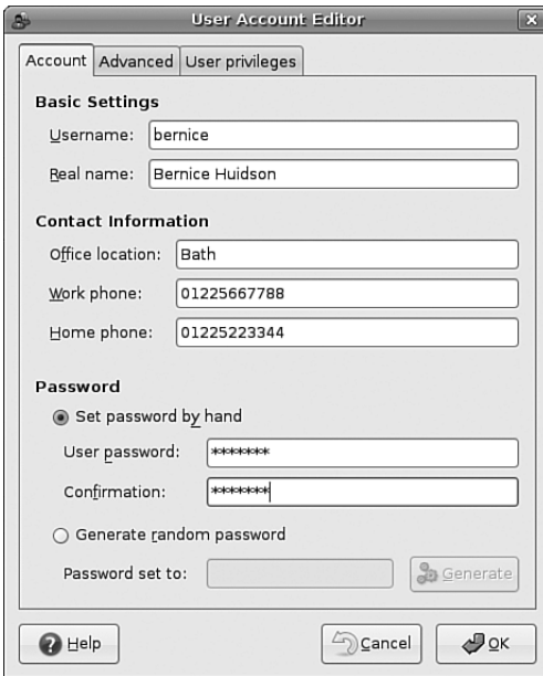
FIGURE 10.2 Adding a new user is simple. The GUI provides a more complete set of commands for user management than for group management.
