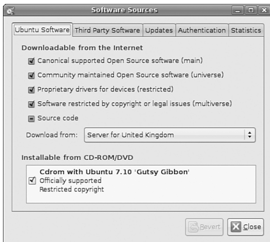
FIGURE 2.2 Enable both Universe and Multiverse repositories to allow access to a huge variety of software for Ubuntu.
