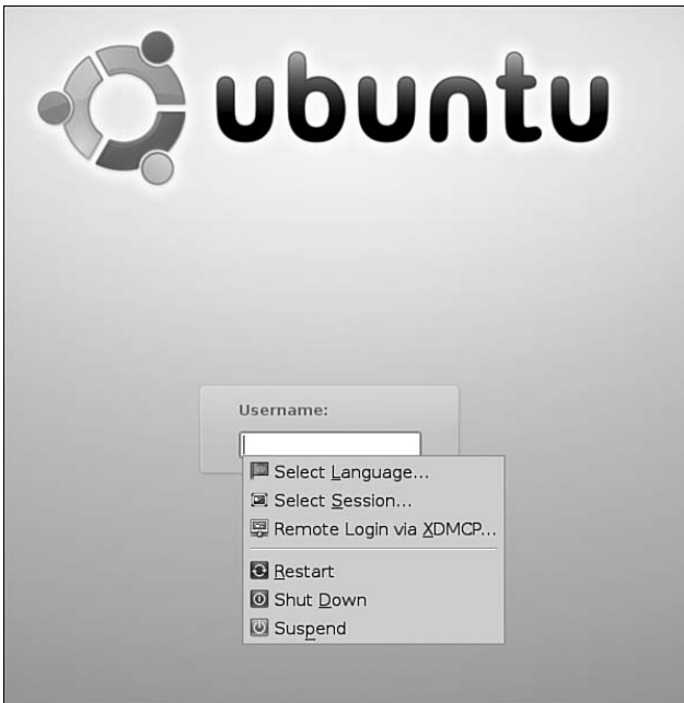
FIGURE 3.9 Use the Select Session option to select the desktop environment of your choice before you log in.
